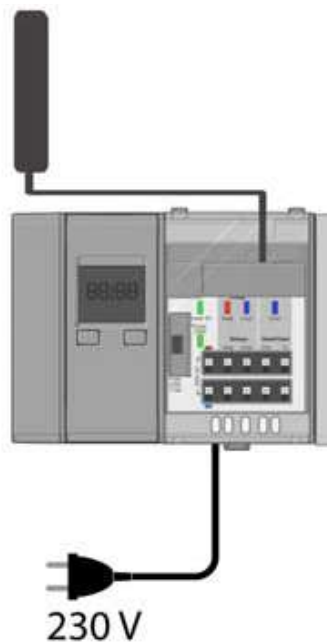
Figure 3: Base module with wireless module for timer module and external antenna
